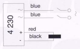
Whole wave rectifier with four terminals for motors with brake power supply on the same terminal block as that of the motor
