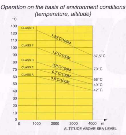
Limits in excess temperatures depending on the altitude at installation for trials carried out at altitudes of less than 1000m, for machinery meant for installation at up to 4000m (coolant temperature 40°C).
