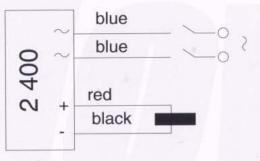
Half-wave rectifier with four terminals for motors with brake power supply on the same terminal block as that of the motor
