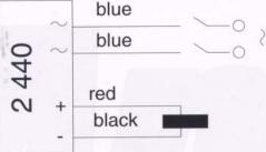
Half-wave rectifier with four terminals (upon request available with five terminals) for motors with power supply separate from that of the motor
