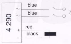
Whole wave rectifier with four terminals (upon request available with five terminals) for motors with power supply separate from that of the motor
