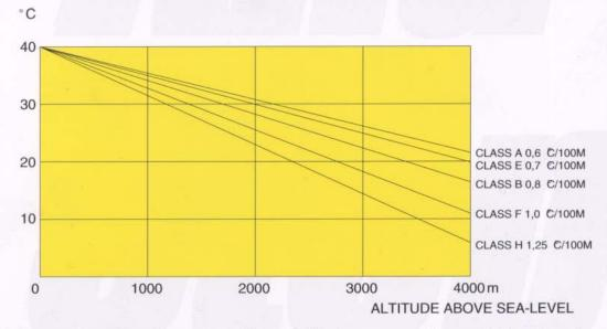
Changes in temperature of cooling air depending on altitude necessary for maintaining the excess temperature, valid up to 100m, also for altitudes between 1000 and 4000m.
